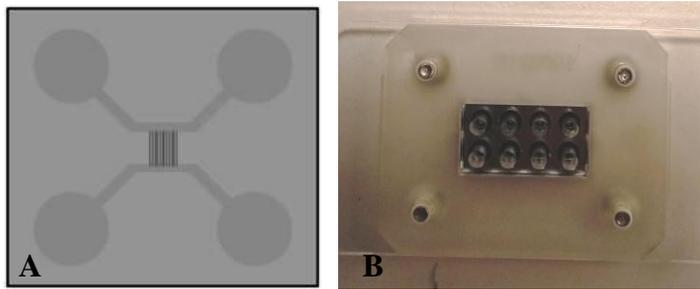
Figure 2.4: A) A schematic view of the micro- and nanochannels connected to the loading chambers. The microchannels are connected to the loading chambers whereas the nanochannels are connected to the microchannels forming an array. B) Image showing the loading chambers in the center which are connected to the micro- and nanochannels. In the device there are two setups of nanochannel arrays and thereby eight loading chambers.
