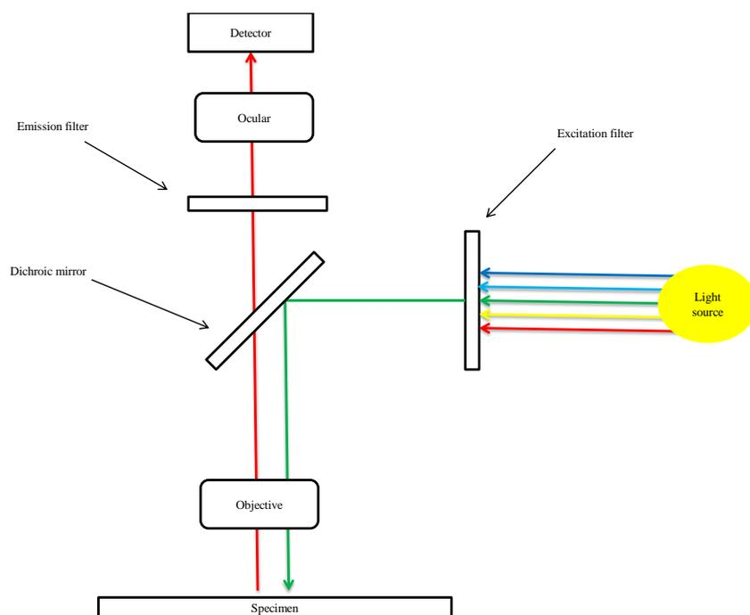
Figure 2.5: The principle of a fluorescence microscope. The components necessary include excitation filter, a dichroic mirror and an emission filter. The specimen will absorb excitation light and emit light of a longer wavelength which is then detected.
