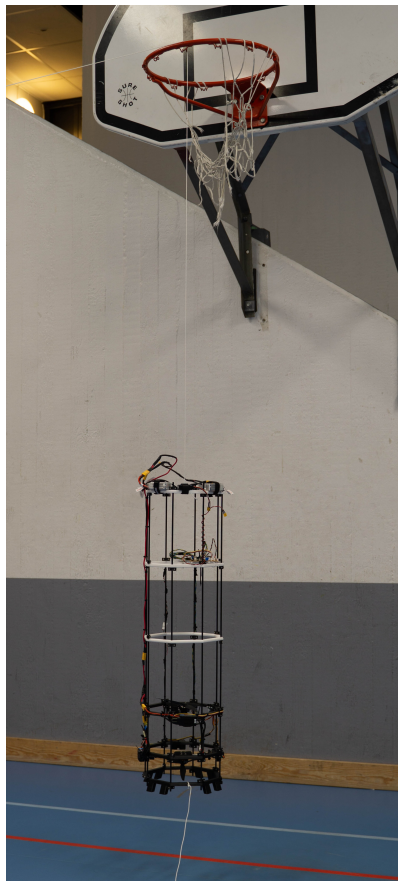
Figure 4.2: Test rig where the model could be saved by pulling on either the upper or lower string.
