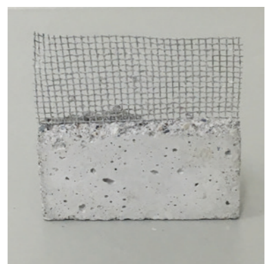
Mesh visible through splitting element.
