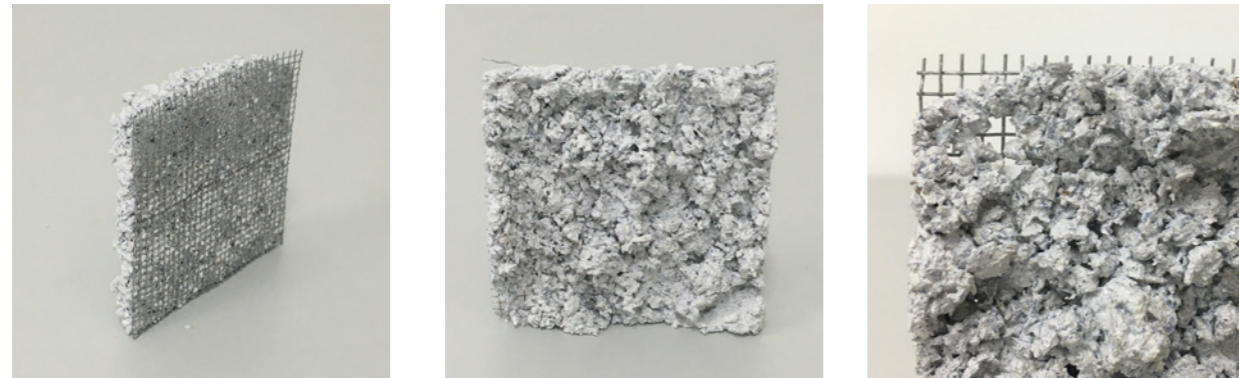
Casted against metall mesh, mix with less water
