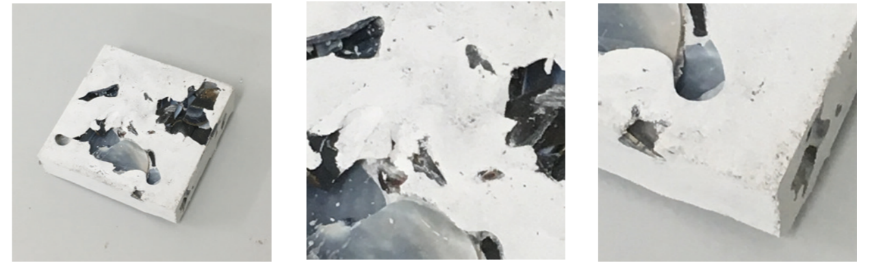
Before: Uncrushed shells where placed in the mold, the result was uncontrolled holes in the cast
