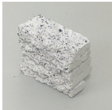
Broken pieces to highlight the rough edge and smooth surface.
