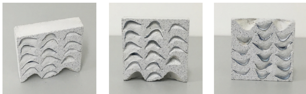
After: Shells in rows, broken shells and sanded with rough paper
