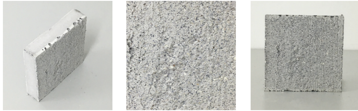
Casted against a rough birch, the result was a relieved, light grey surface
