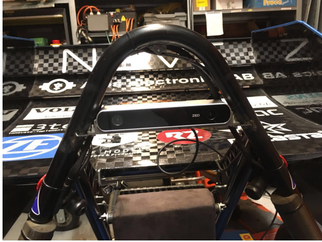
Figure 3.1: This is a stereo camera mounting under the main hoop of the vehicle.
