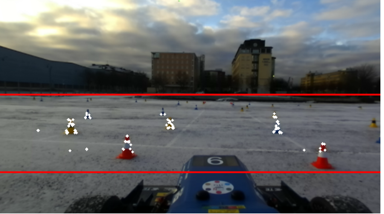
Figure 2.12: ORB detection result of an example frame in the testing track. The white spots in the image are keypoints detected by ORB. The detection is limited within the region of interest (the area between the two red lines), where most cones are located.
