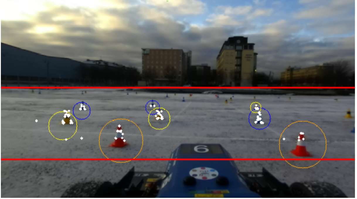
Figure 3.5: The result of the supervised detector in an image captured on a sunny winter morning.
