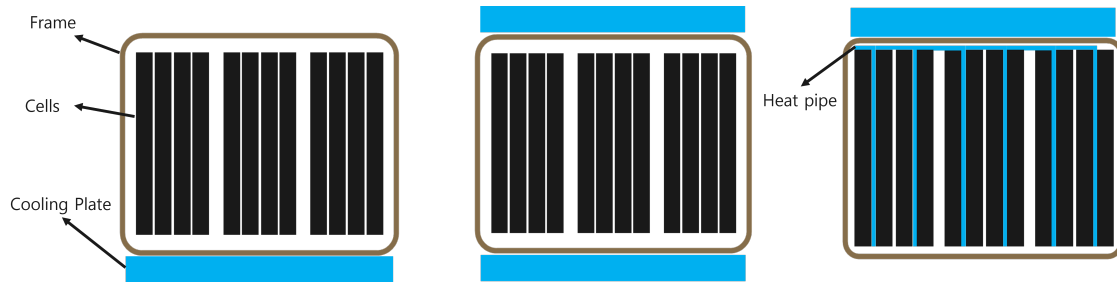
Figure 3.15: Cooling strategies for designs A, B, and C
