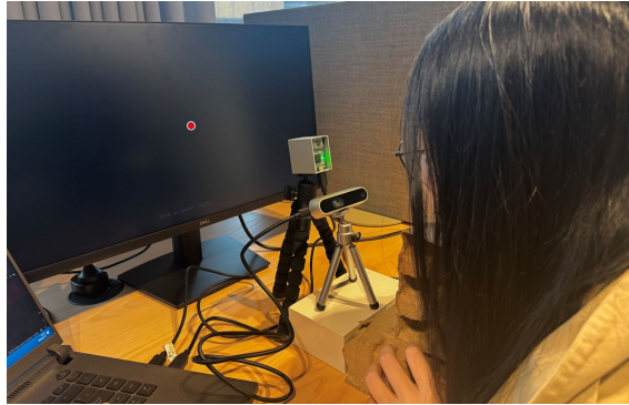
Figure 3.4: Laboratory geometry for synchronous radar-camera-stimulus acquisition.
