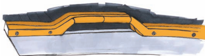
PICTURE 3.47 - RAISED SPLINE-CENTRE HANDLE CONCEPT. REGNER (2012).
