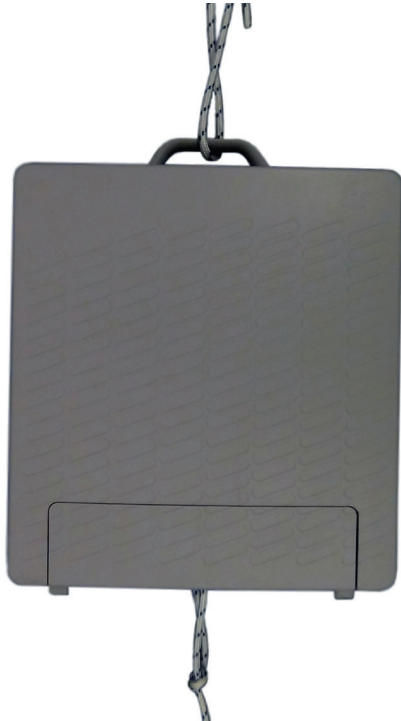
PICTURE 2.14 - ROPE CONNECTED TO RRUS 11. REGNER (2011)
