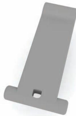
PICTURE 5.29 - HOLE IN THE ARMS FOR CONNECTION OF SPRINGS. REGNER (2012).
