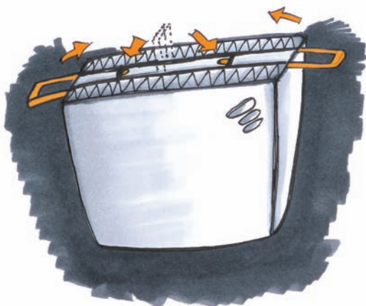
PICTURE 3.17 - SLIDING AND FOLDING ALONG THE TOP CONCEPT. REGNER (2012).
