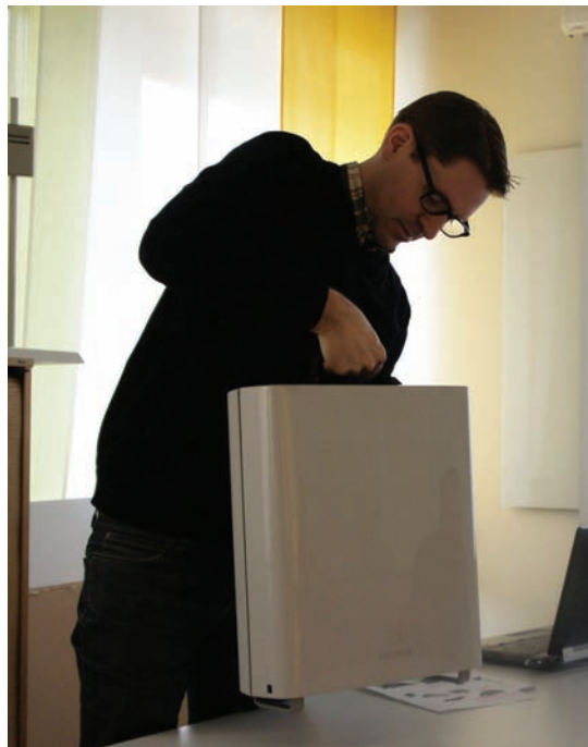
PICTURE 5.56 - ERICSSON AB PRODUCT HANDLED AND FITTED WITH REDESIGNED HANDLE MOCK-UP. REGNER (2012).
