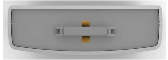
PICTURE 5.25 - CARRYING FEATURE FITTED TO ERICSSON AB RRUS 12 FROM ABOVE. REGNER (2012).
