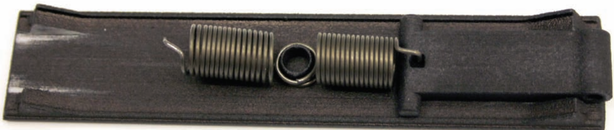
PICTURE 5.48 - SPRING ASSEMBLED TO THE LID AND ARM MOCK-UP. REGNER (2012).
