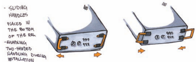
PICTURE 3.14 - SLIDES FROM THE BOTTOM CONCEPT. REGNER (2012).
