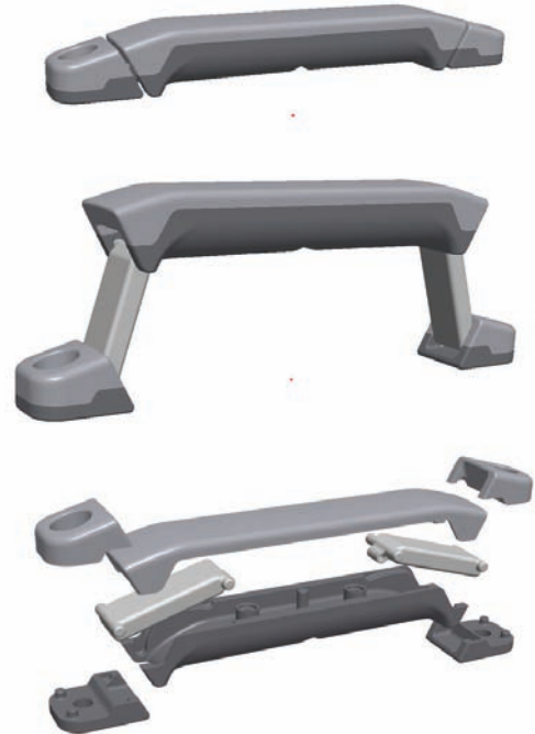
PICTURE 5.57 - PATENTED HANDLED, EXPLOSION VIEW. KALLIN (2013).
