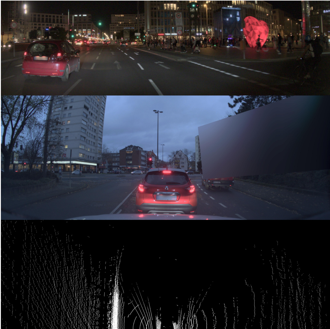
Figure C.2: A selection of high entropy frames on ZOD 2 [1]. The top image shows an image with many occluded pedestrians at night. The middle image shows an image with a weird blur. The bottom image shows a LiDAR point cloud where the data from the main Velodyne VLS128 LiDAR is missing.
