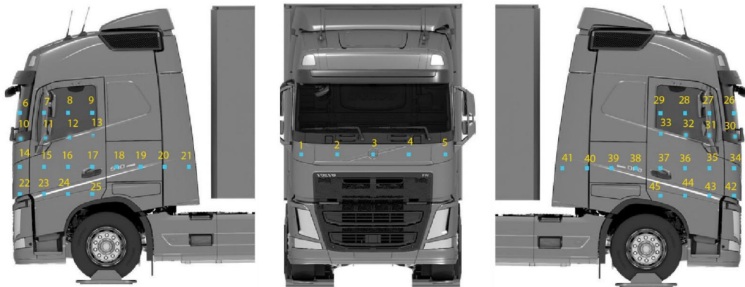
Figure 5.11: Pressure tap positions on cab of Configuration 1, marked with numbers. Figure taken with permission from [6].
