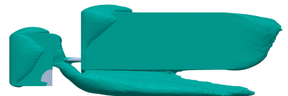
Figure 4.30: Iso-surfaces of separation where C_{p,tot} = 0 . Left column: isometric view; center column: bottom view; right column: left-side view.
