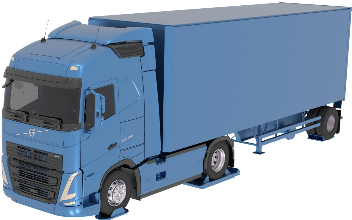
Figure 5.1: FH truck with wind tunnel mountings and the shortened trailer.
