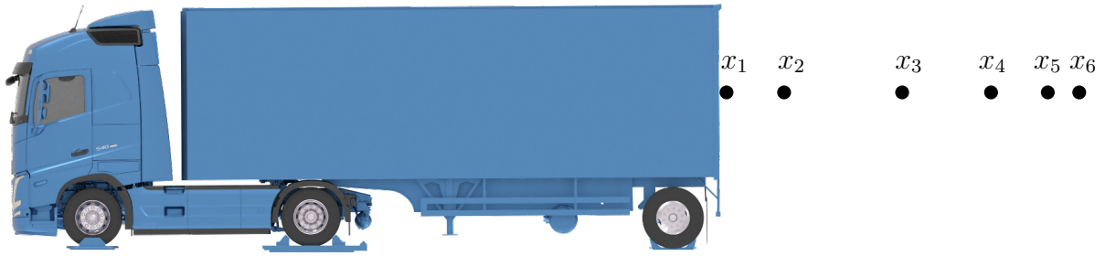
Figure 5.33: Schematic of the six pressure probe positions x_1 – x_6 in the trailer wake relative to the trailer rear face, at distances 0.1 m, 0.8 m, 3.1 m, 4.6 m, 5.6 m, and 6.1 m, respectively. All probes are placed on the y = 0 plane, forming a straight line in the streamwise direction.
