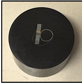
Figure 3.2: shows a figure of the exposed Fe sample after the preparation for SEM imaging.
