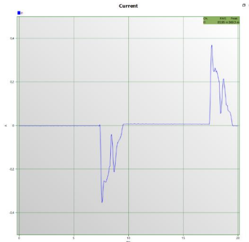
Figure 34a. White light's current wave with THDI = 148.45%
