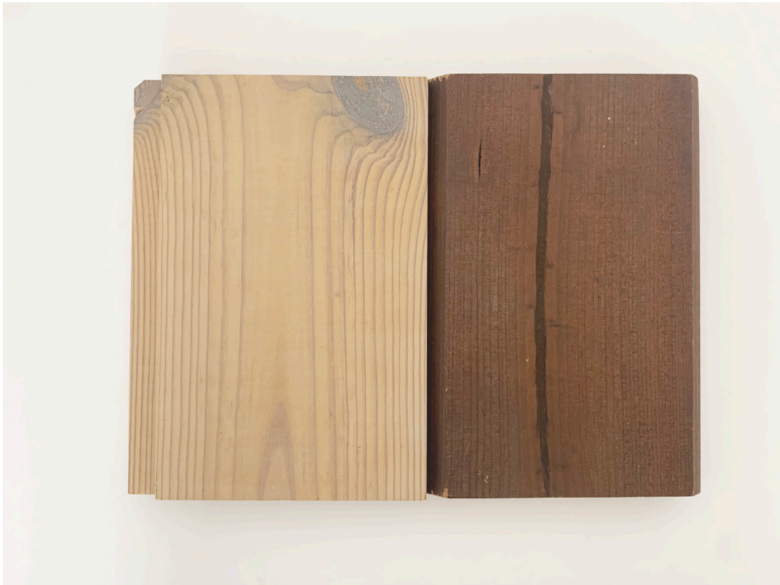
The impregnated fire proofed wood. The light one to the left is used on the facade and the dark one to the right is used on the window frames.
