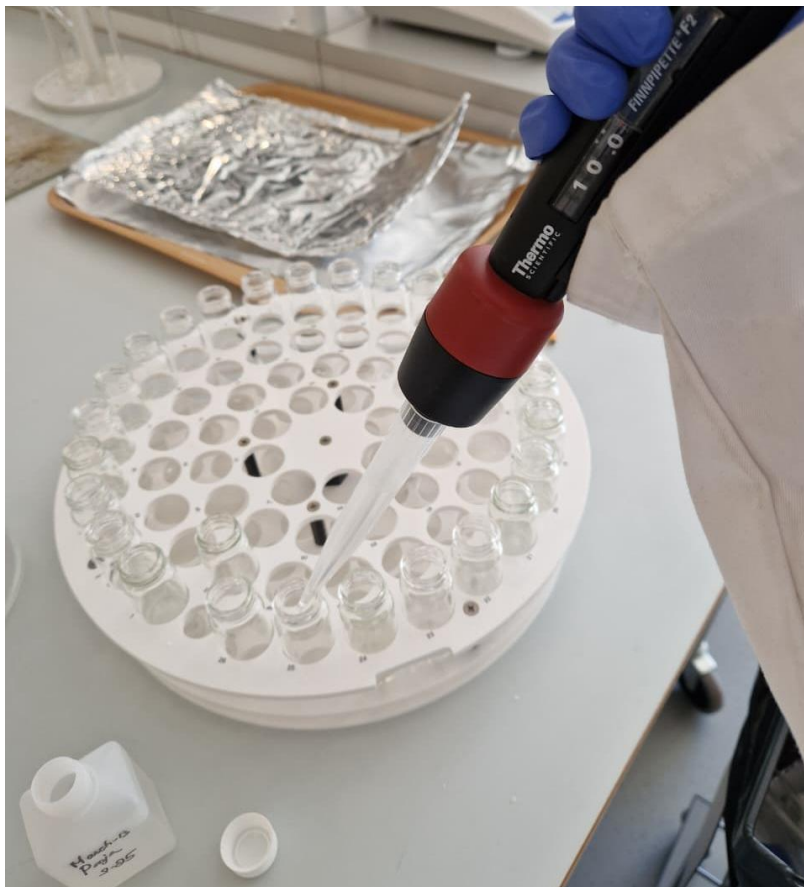
Figure 21: Preparing samples for TOC analysis 20ml distilled water with 20ml water sample
