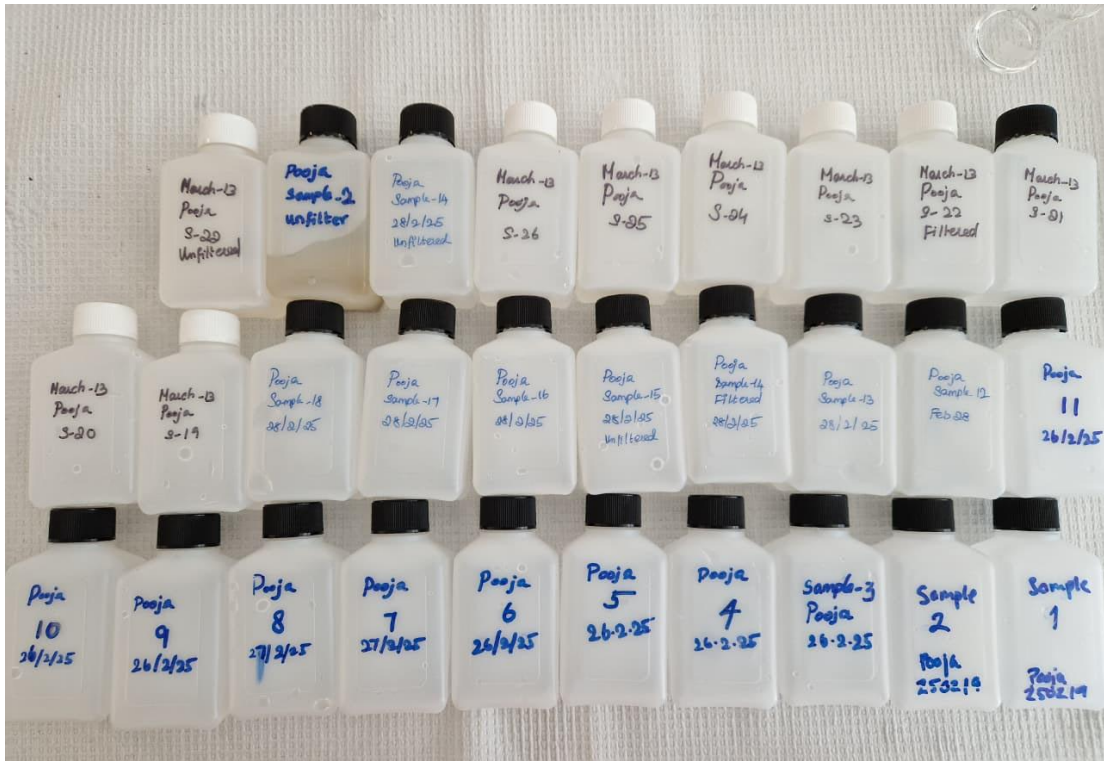
Figure 20: Defrost frozen water samples for TOC analysis. samples were marked with name, sample number and date of collection.
