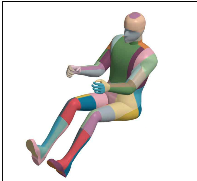
Figure 5: 58 surfaces as required by the Fiala thermal model
