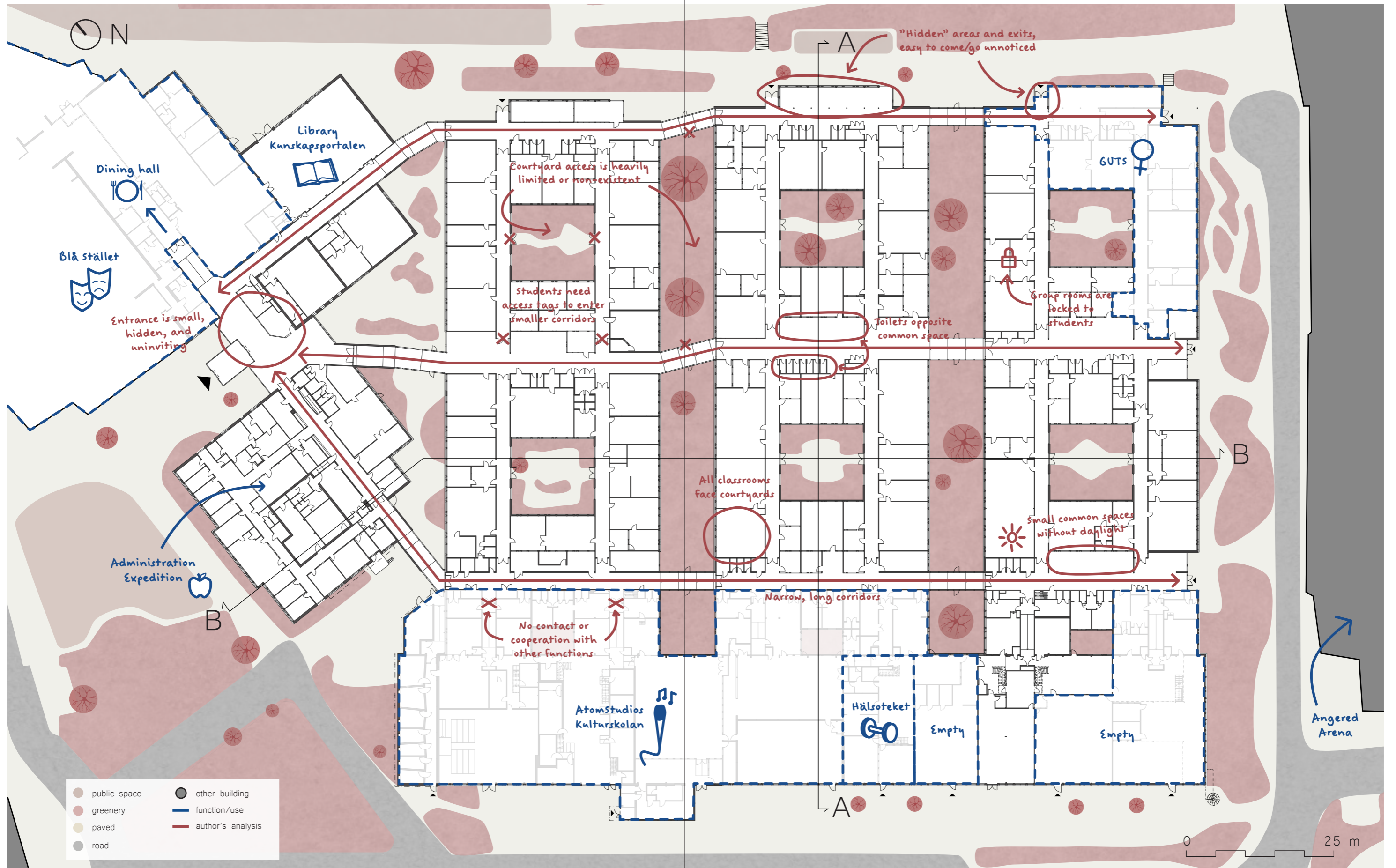
Figure 6. Ground floor of Angeredsgymnasiet, scale 1:600. The blue annotations on the plan show the different functions while the red annotations show my analysis of the building based on site visits, interviews, and mappings. The main noteworthy aspects are the long and dark corridors that feel cramped and unpleasant, as well as the lack of common spaces where the students can spend their breaks.
