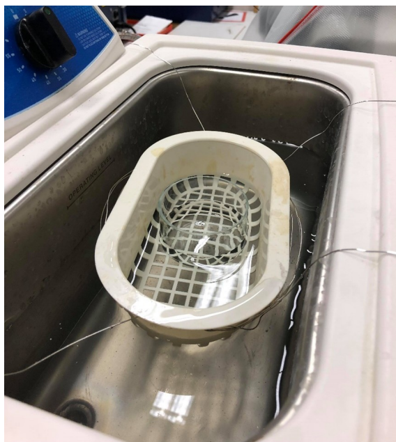
Figure 3.7: Cage setup for sample sonication in Branson 3800 ultra-sonic bath.
