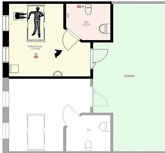
Figure 3.1: A schematic birds-eye view of the patient room relative to the corridor and bathroom.
