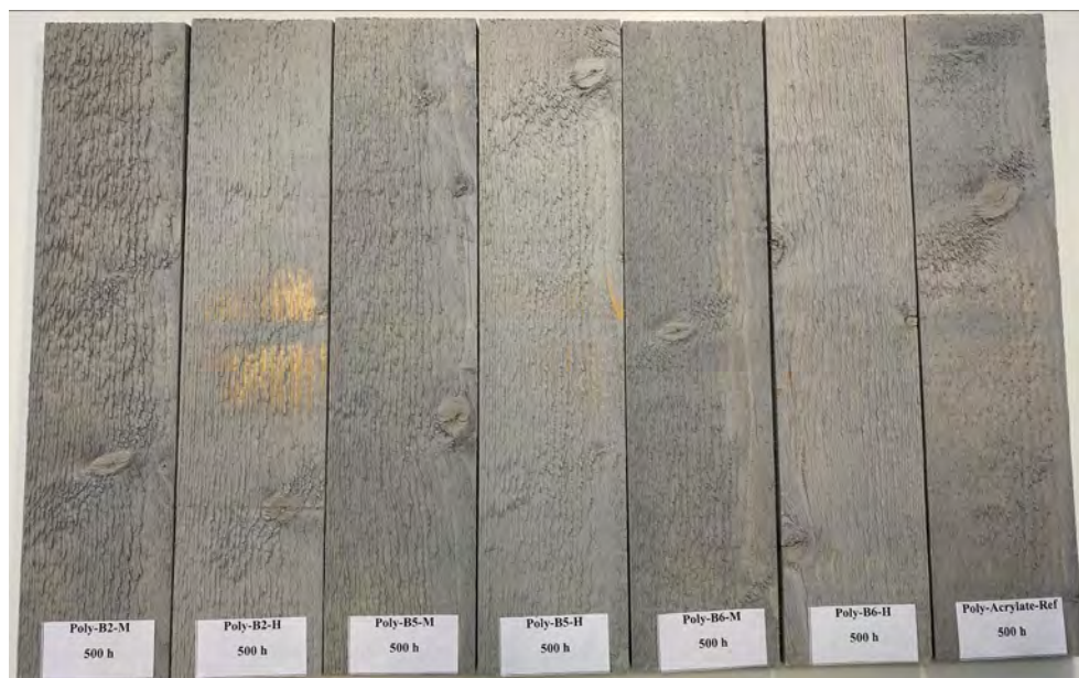
Figure 5.57: QUV accelerated weathering for all polybinder paints for 500 h
