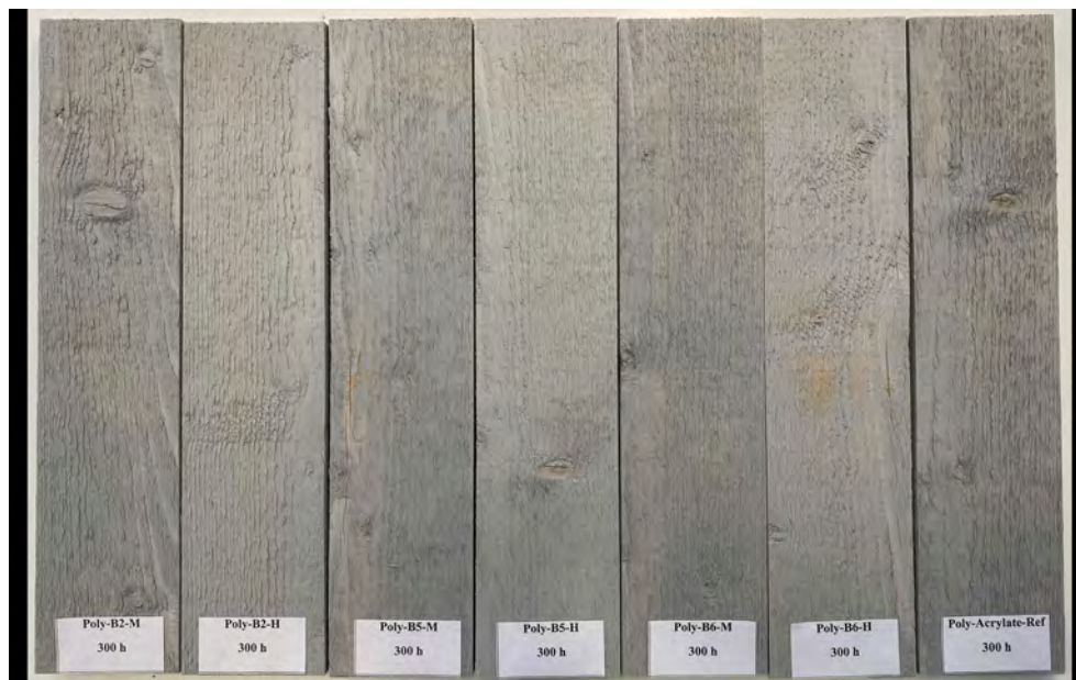
Figure 5.56: QUV accelerated weathering for all polybinder paints for 300 h
