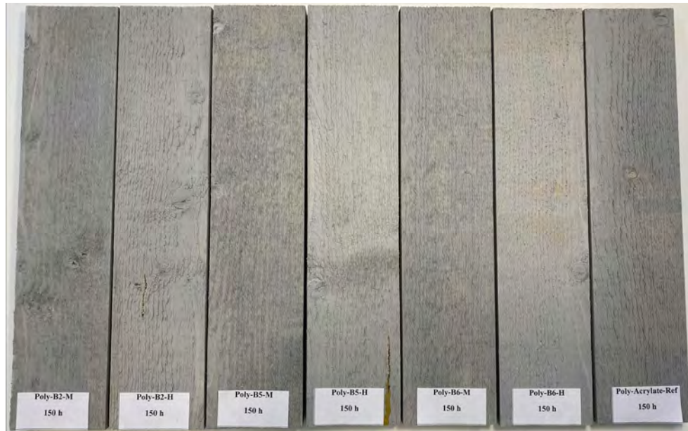
Figure 5.55: QUV accelerated weathering for all polybinder paints for 150 h.
