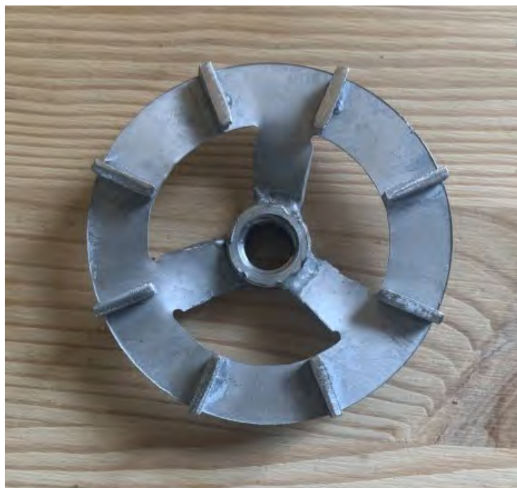
Figure 3.2: Lenart disc used in the dissolver for paint production.
