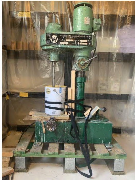
Figure 3.1: Dissolver and construction used for paint formulation.
