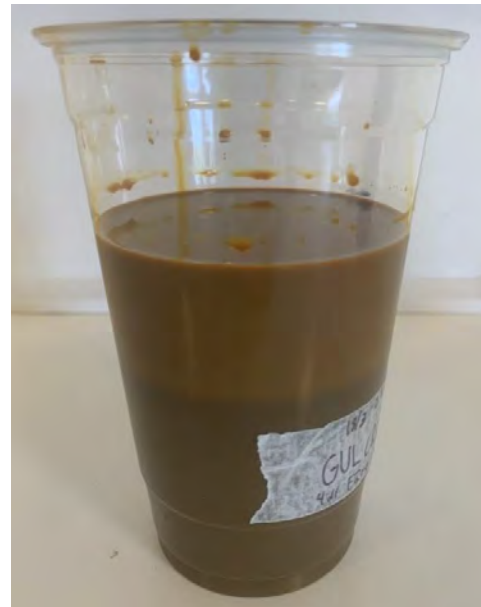
(b) Pigment separation in the stability test for Yellow Acrylate 20% .
