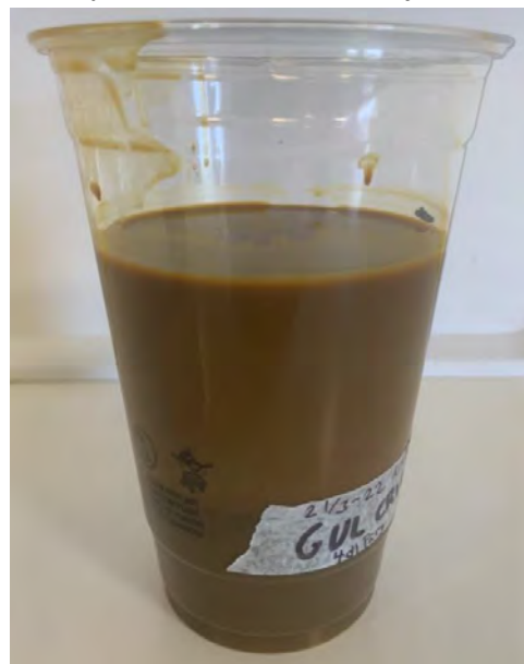
(d) Pigment separation in the stability test for Yellow Acrylate 30% .
