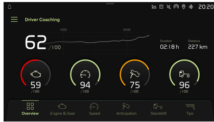
Figure B.2: View the overall accumulated score of eco-driving, and view of key performance indicator's (KPI's) gauges
