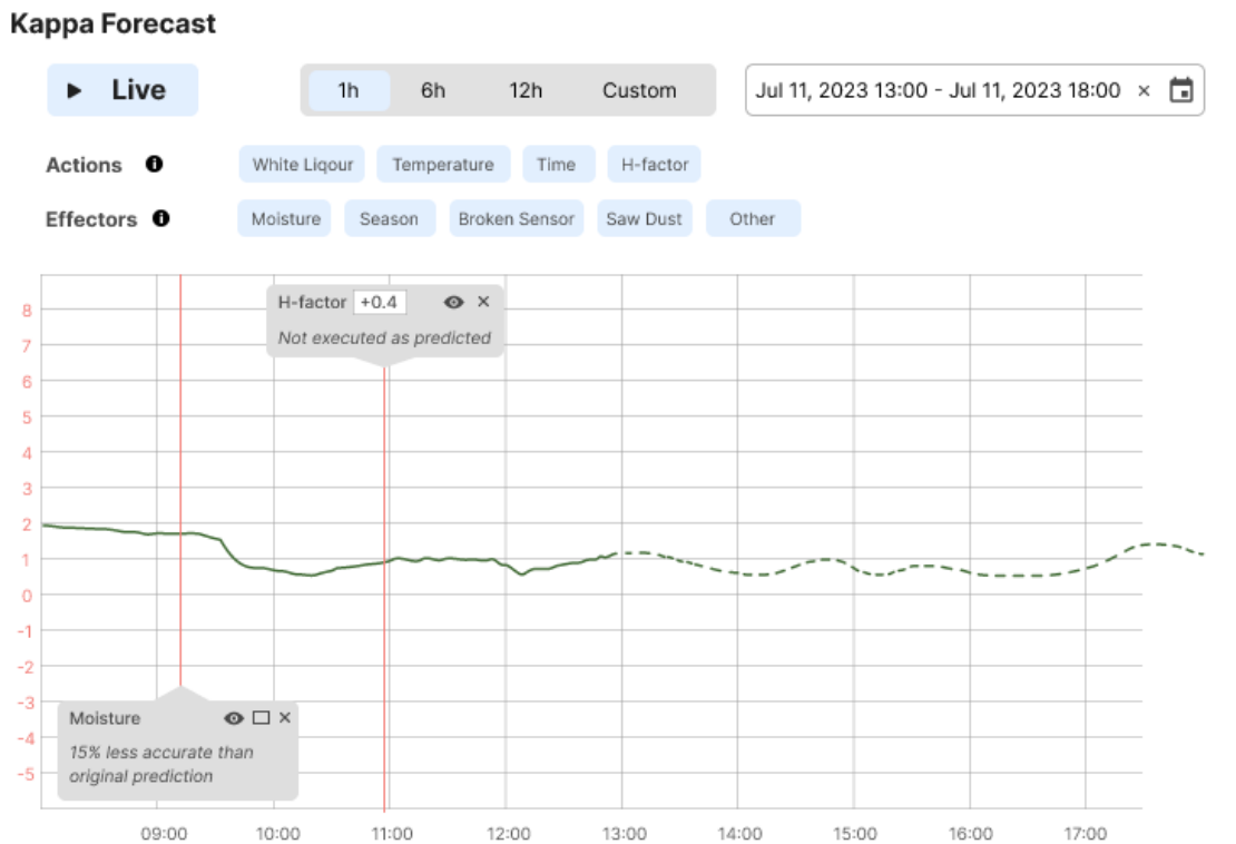
Figure 6.8: The IPG component showing the post-event prediction accuracy when the prediction was inaccurate.
