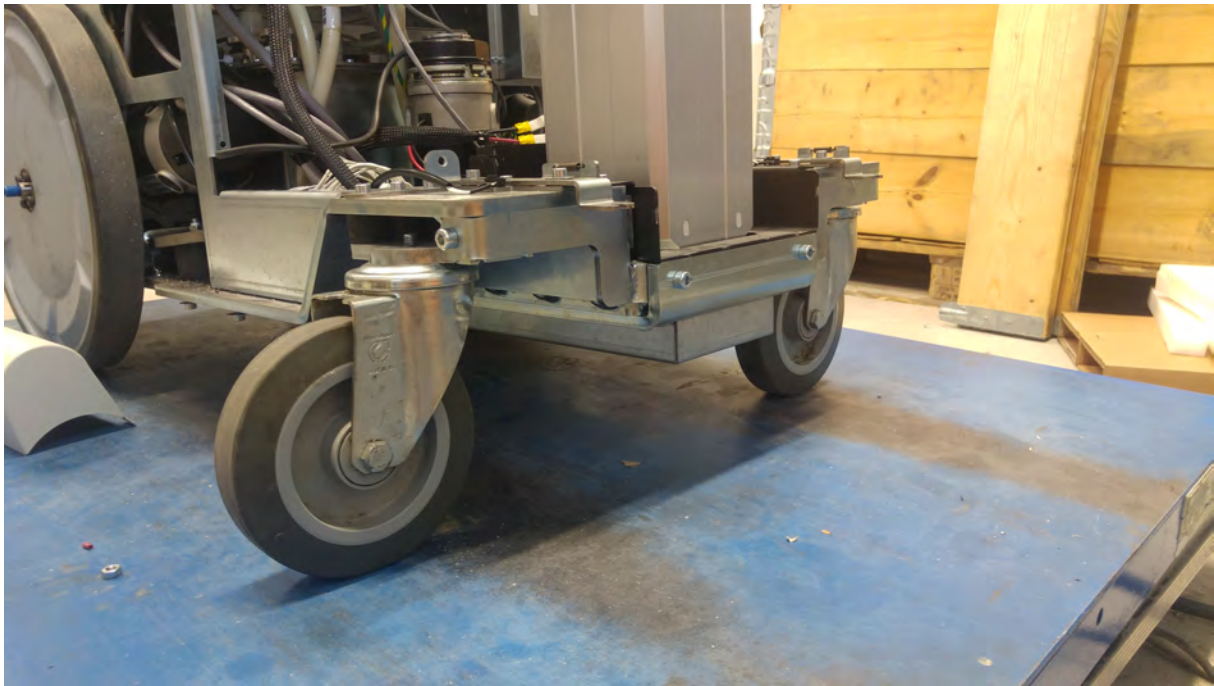
Figure 6.12: The front wheels place in an disadvantageous position
