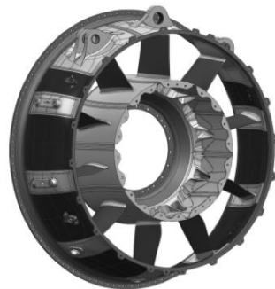
Figure 18. Complete assy with H-sectors and case plates
