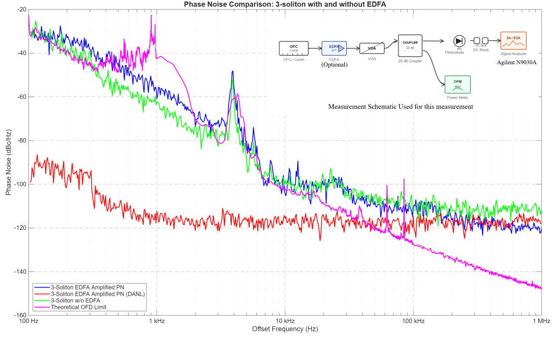
Figure 4.5: Phase noise comparison at 49.921 GHz of a 3-soliton state without the EDFA (green) and with the EDFA (blue) inserted in the optical output path, measured using the Agilent N9030A PXA Signal Analyzer. The red trace plots the displayed average noise level (DANL) of this measurement. The EDFA improved the high-offset noise floor but degrades close-in phase noise below 1 kHz, where comparison against the theoretical 2-point OFD limit (pink) matters most. Shown in the inset is the measurement schematic used.
