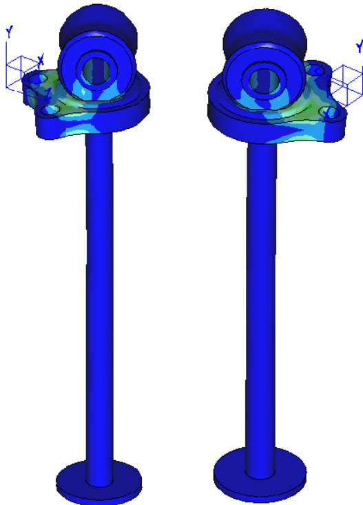
(c) FEM analysis of the detailed design version 2 - Suspension plate analysis. The maximum allowed stress is set to 500 MPa
