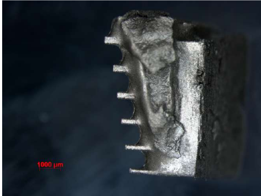
Figure C.1: Residual feedstock remaining on a component after the de-caking stage, caused by premature polymer binding within the unhardened material.
