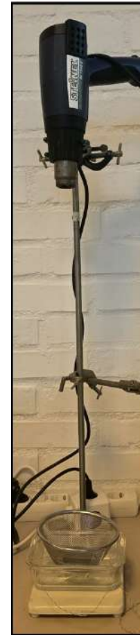
Figure 9: Heat gun stand during de-caking with a glass container to catch excess feedstock.
