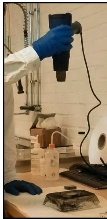
Figure 7: Initial de-caking setup used, where heat was applied manually using a handheld heat gun.
