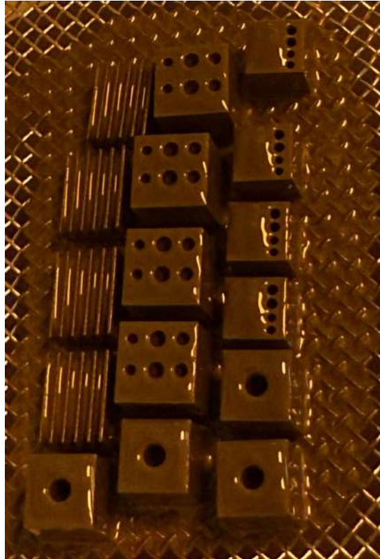
Figure 34: Components without build plate, unrestrictive flow through channels.
