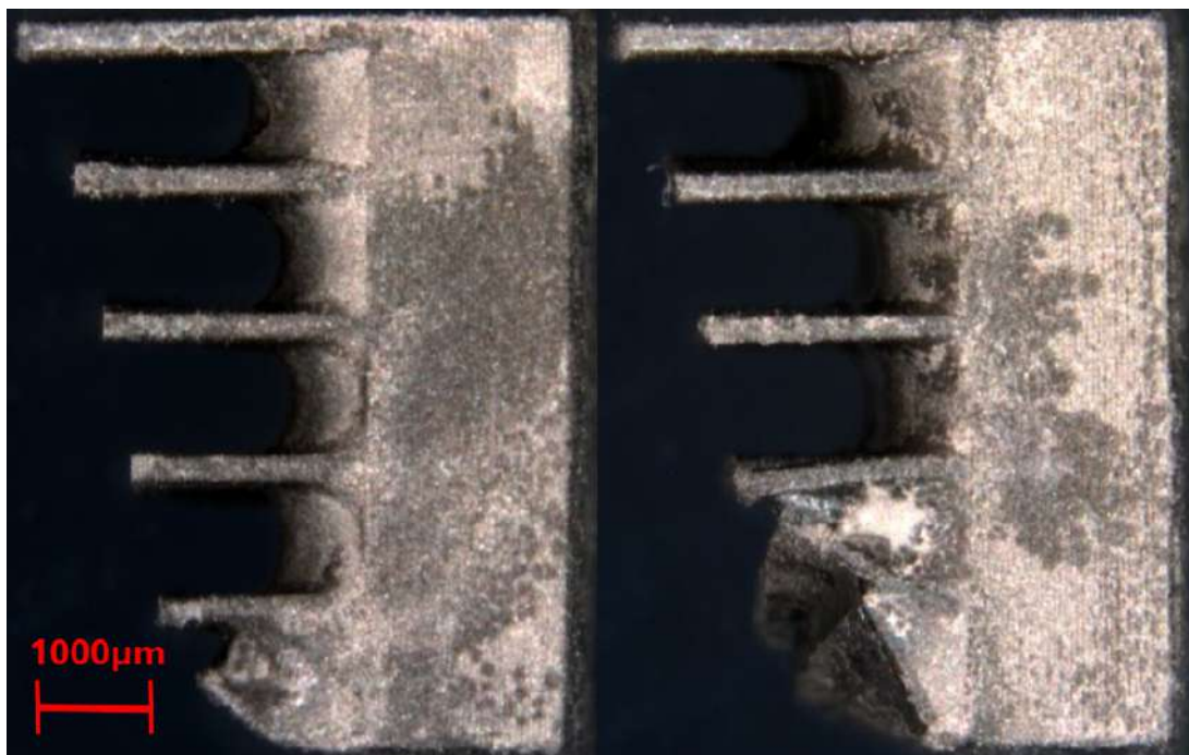
Figure 27: C-components cleaned with airbrush. Damage to the fins can be seen in the thinnest and shortest fins for both specimens.
