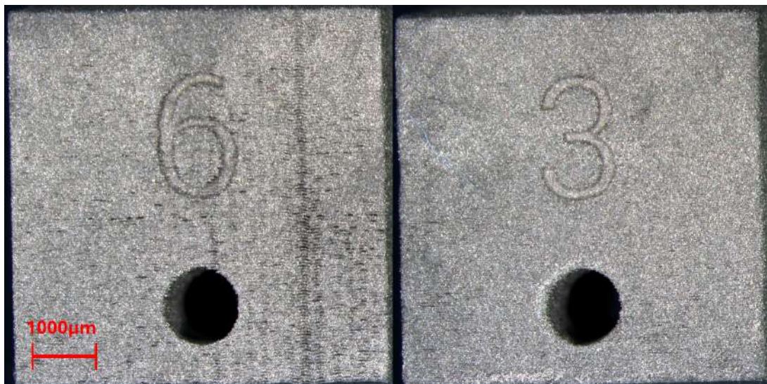
Figure 51: Side views of the D-component shown in Figure 50, displaying two of the cleaned outlet channels connected to the internal junction.
