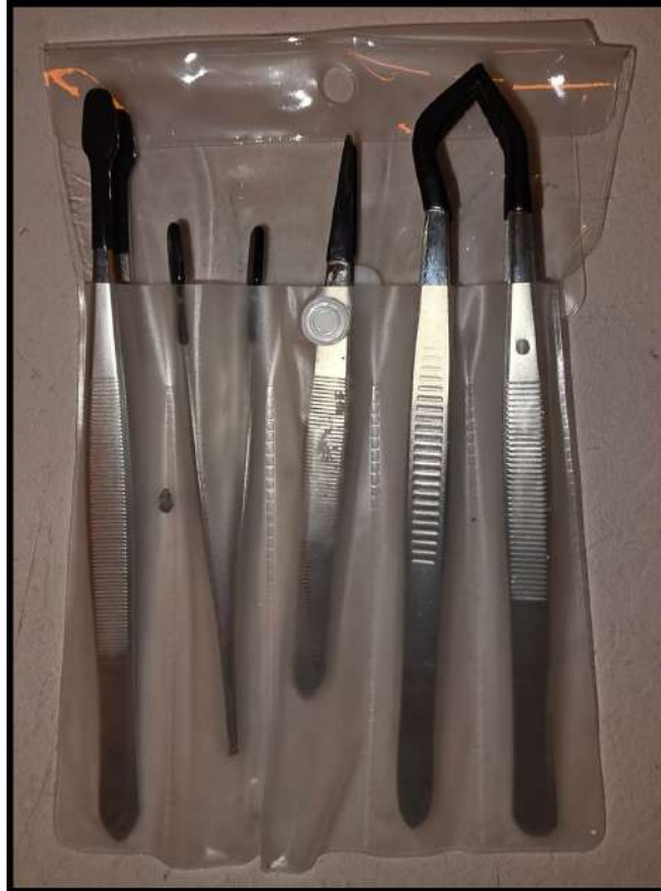
Figure B.5: Rubber-coated metal tweezer set used for manual handling of components.
