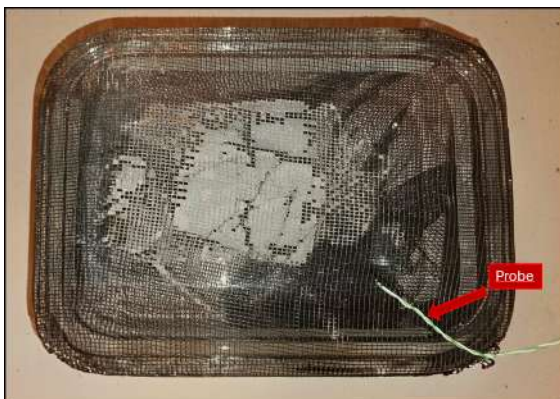
Figure 8: Placement of temperature measuring probe during tests
