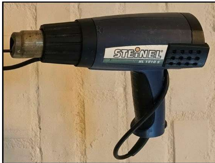
Figure B.1: Heat gun used for de-caking and heating of the components.
