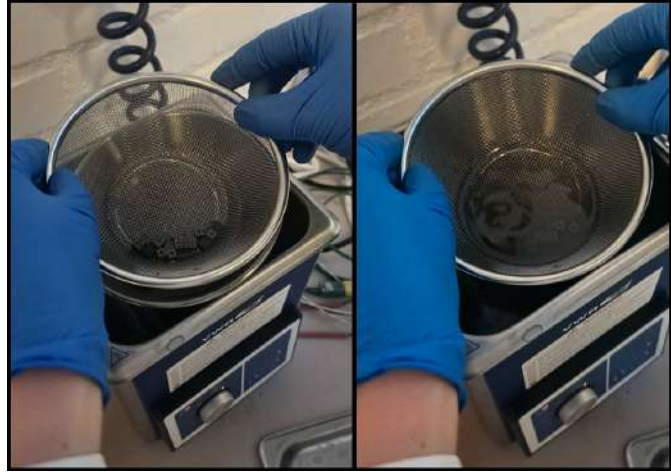
Figure 15: Ultrasonic cleaning setup used. The right side shows the components submerged in heated IncuSOL, while the left side shows removal of the strainer to remove one of A-, B- and D-component.
