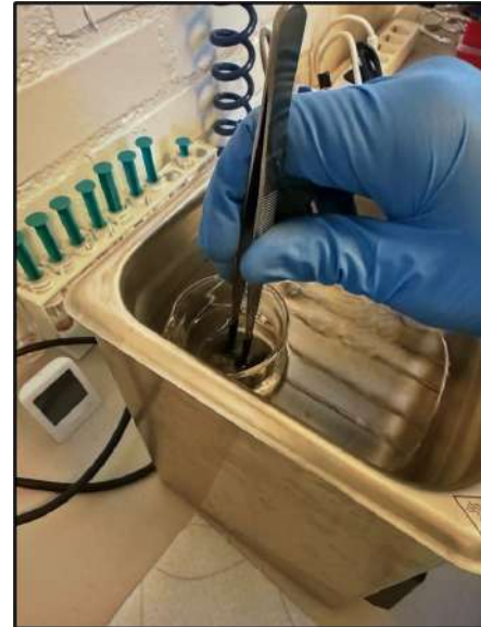
Figure 12: Short intermittent ultrasonic cleaning cycles performed in heated IncuSOL.
