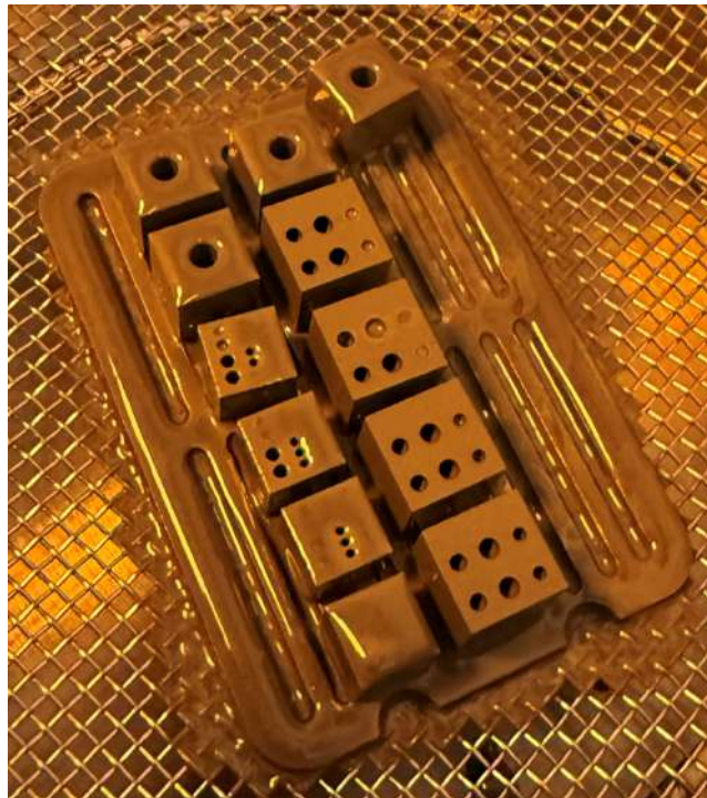
Figure 29: Build plate after initial heating, note how clearing of channels corresponds with placement on the build plate.
