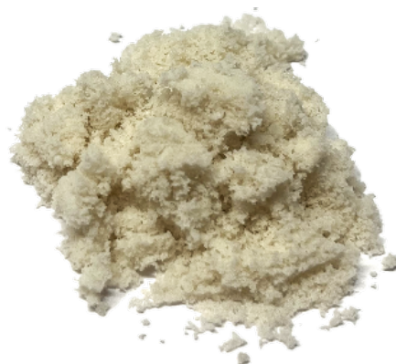
(c) Crystals obtained from run 1.7 with bleed stream from Mill 2 at 32 °C, believed to be Product A.
