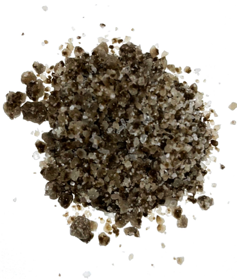
Figure 4.1: Solids found in can SII before run 1.3.
