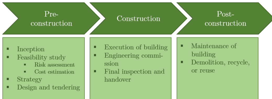
Figure 2.1: Three phases of the construction process, based on an interpretation of Boverket (2021b) and Fewings & Henjeweale (2019).
