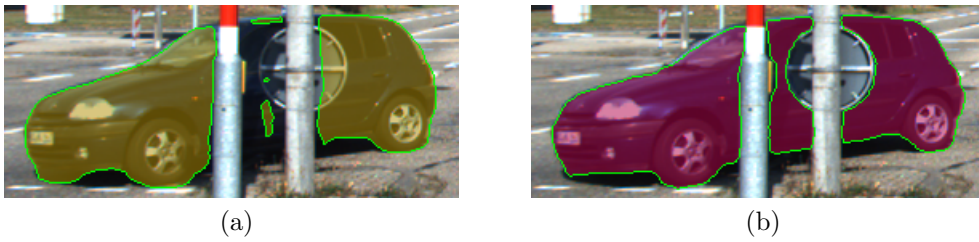
Figure 4.4: A segmentation mask, for which the model struggled with detecting the car due to occlusion, in (a). The corresponding ground truth mask in (b).
