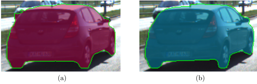
Figure 4.3: A segmentation mask where part of the background was wrongfully predicted as car in (a). The corresponding ground truth mask in (b).
