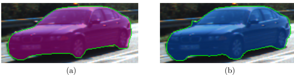
Figure 4.2: A segmentation mask, in which the side mirror was not detected, in (a). The corresponding ground truth mask in (b).
