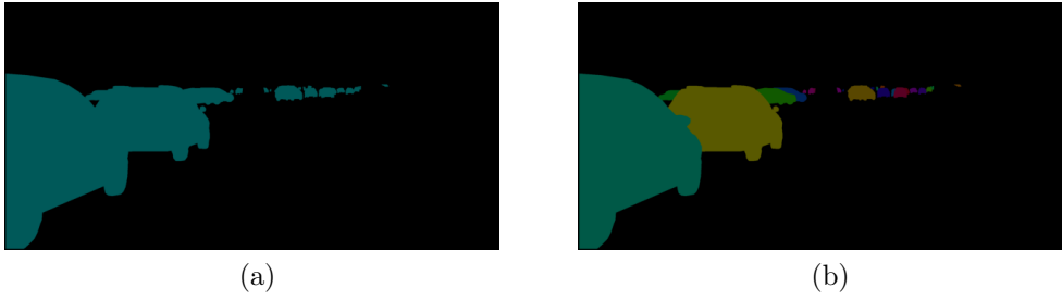
Figure 2.1: Masks from the Cityscapes dataset [38] produced with semantic (a) and instance (b) segmentation with the classes background and car. Different cars are segmented as separate objects and illustrated with various colours when instance segmentation is applied, while all cars have the same label and colour for the semantic segmentation.
