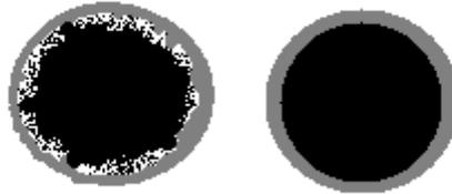
**Figure 9** – Schematic cross section of the silver paint wetting of sanded (left) and non sanded (right) strands.
