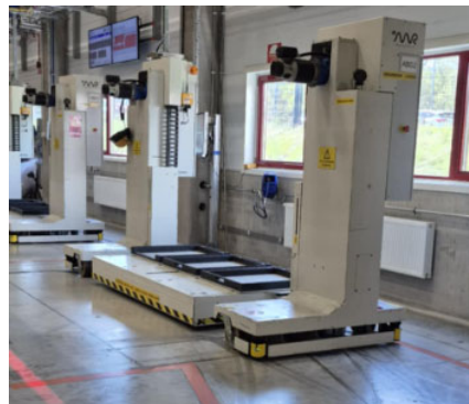
Figure 4.14: AGV used for delivering batteries for electric vehicles to the assembly line
