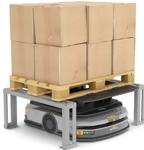
Figure 5.2: Underdrive AGV lifting a unit load. Support structure allows AGV to lift the unit load [33]. Reprinted with permission.
