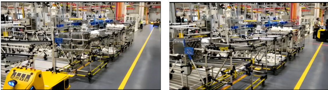
Figure 5.11: An AGV using Karakuri solutions to unload a tugger train at PoU [Volvo's internal documents]
