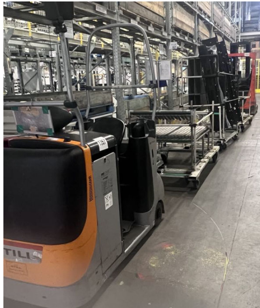
Figure 4.7: Tugger train used for Synchronous deliveries
