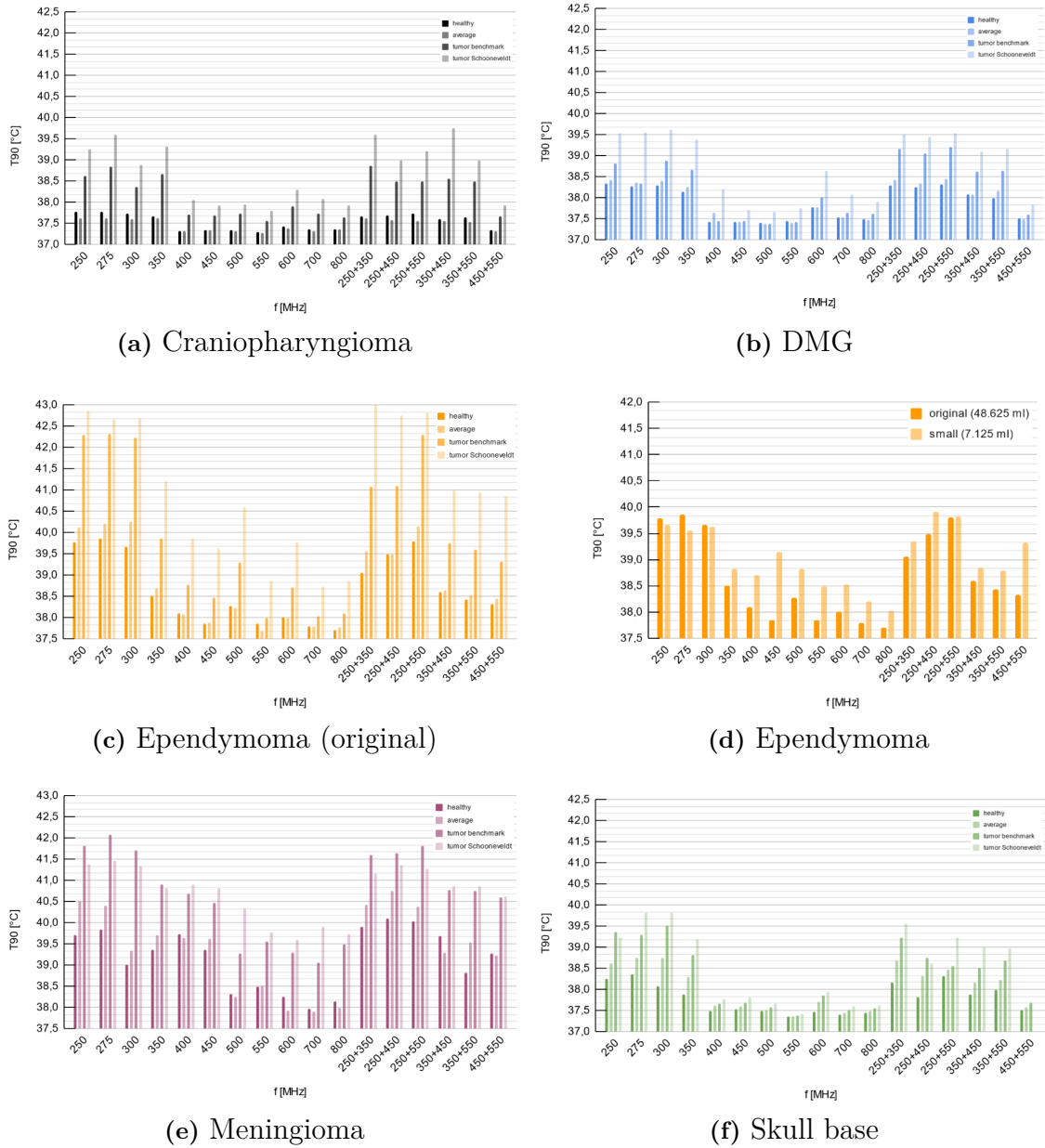
Figure 5.4: T_{90} at single frequencies and frequency combinations for each target. (d) show the T_{90} for healthy tissue parameters using the original (left bars) and smaller (right bars) ependymoma. Note that the y-axis runs between 37.0 – 42.5 °C for (a)-(b), and between 37.5 – 43.0 °C for (c)-(f).
