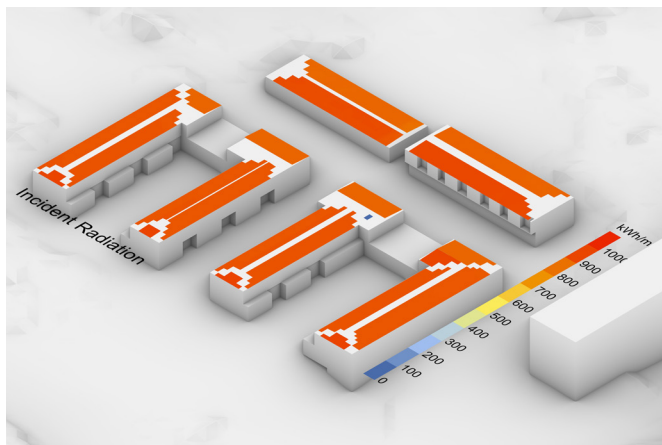
Figure 39. Proposal 1 with PV over the existing roof
