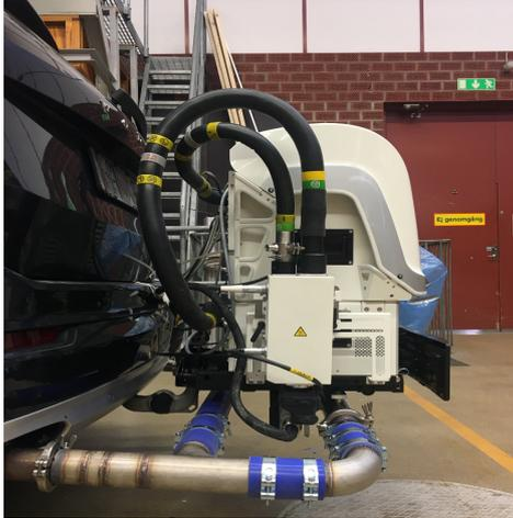
(a) PEMS mounted on towbar with its probe connected to the modified exhaust pipe
