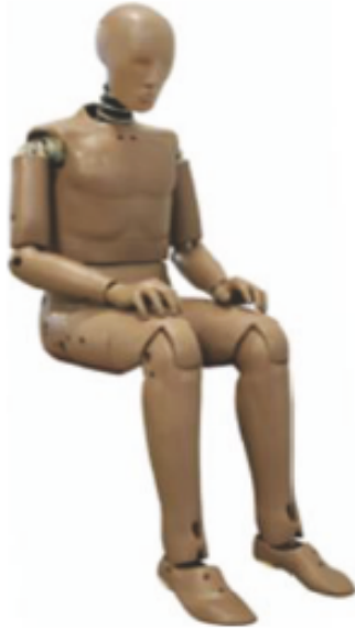
Figure 1.2: Hybrid III 50th percentile male dummy model used for frontal impact test.
