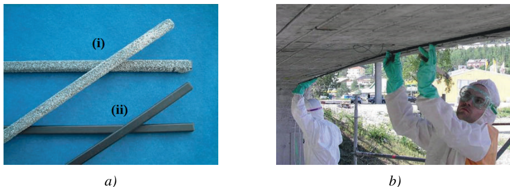
Figure 4.1 a) NSM-rods with (i) quartz sand compared to (ii) ordinary NSM-rods. b) Work performed using NSM-rods (Täljsten, Blanksvärd and Sas, 2016).
