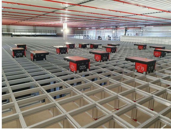
Figure 3.2: Cube-based ultra-high-density automated storage and retrieval system with robots operating on a grid structure (Euku, 2025)
