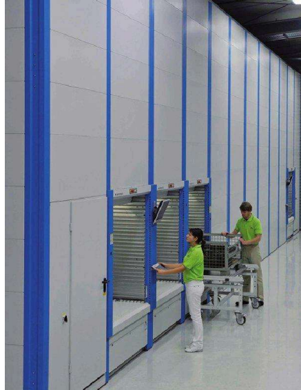
Figure 3.5: Automated vertical lift module (VLM) warehouse system utilizing internal tray retrieval mechanisms (WindyPrints, 2010)
