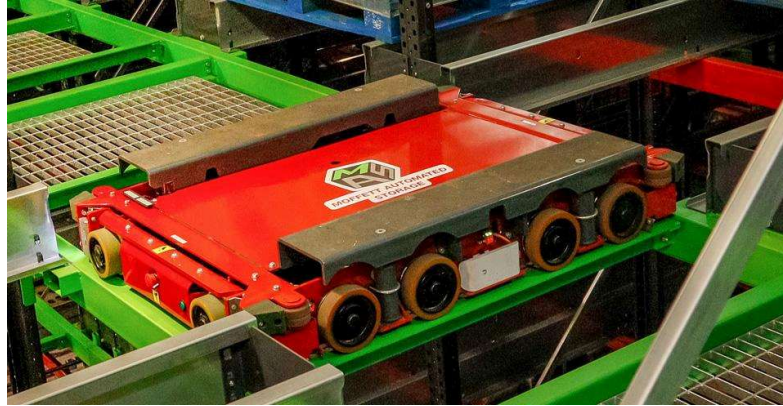
Figure 3.3: Autonomous storage shuttle vehicle operating inside an automated racking matrix (Moffett, 2020)
