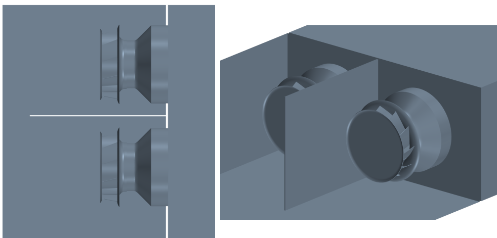
Figure 3.15: Top view (left) and isometric view (right) of the AHU with the straight wall concept
