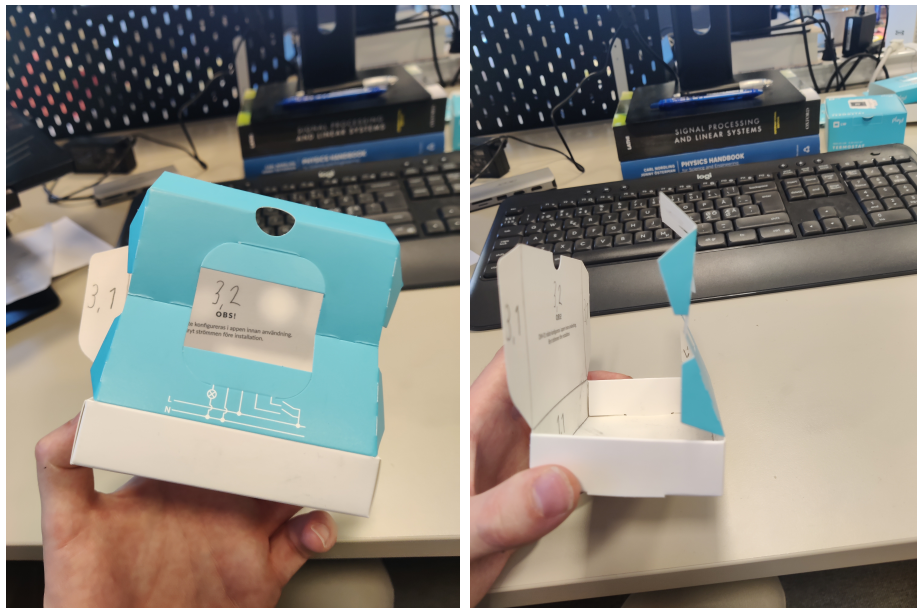
Figure 5.7: The front and side view of the packaging with side panels folded and insert bended to be able to slot into the packaging (Authors own images).
