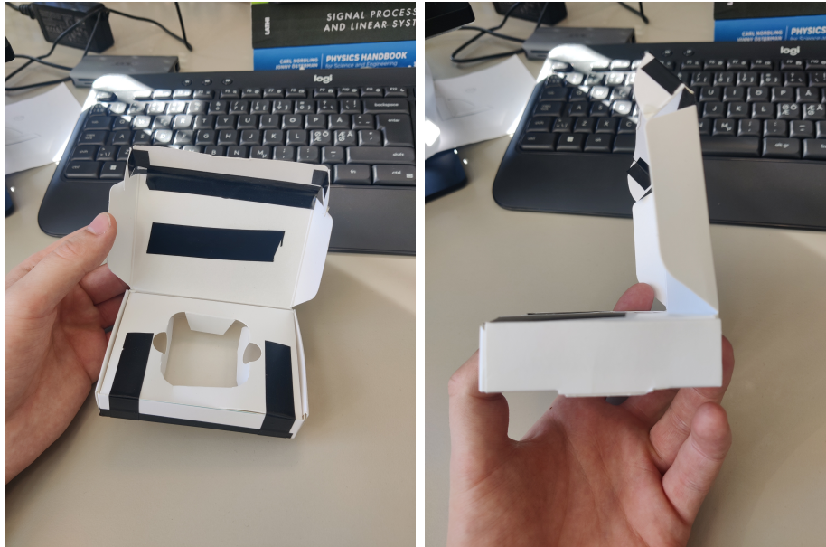
Figure 6.11: The front and side view of the modified packaging. This packaging has removed the sleeve in favor of an extra panel with side panels use to lock down the top lid. The insert is replaced with an insert that is not angled allowing for an easier motion of folding. (Authors own images)
