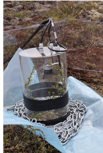
(b) Chamber with chains placed around it, on the plastic skirt.
