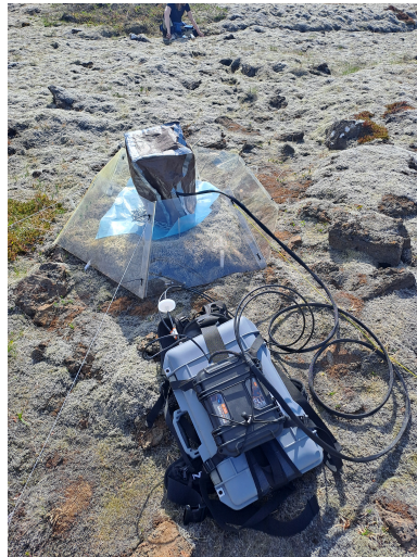
(c) Licor instrument in the foreground and a blackout bag on top of the chamber placed in an OTC in the background.
