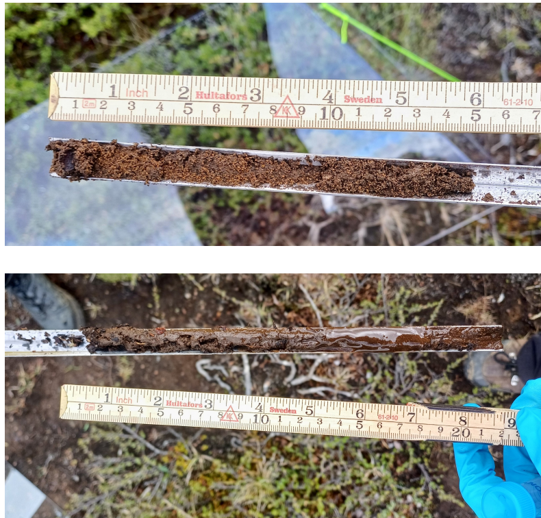
Figure 3.6: Example of two soil samples taken at the same day from different plots with visually differing soil moisture.
