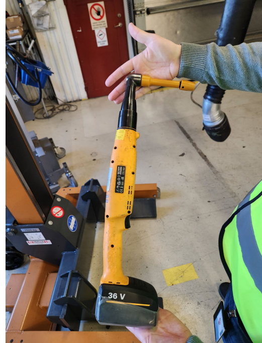
Figure 1.3: Battery-powered torque wrench presently used for fastening
