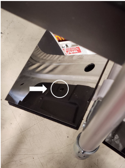
Figure 6.11: The operator's view for Mirror Align, with the area of interest circled in red
