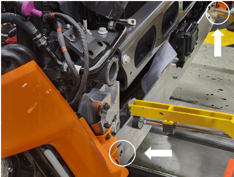
Figure 3.1: Additional bolts of the FUP concealed by the bumper for the FML
