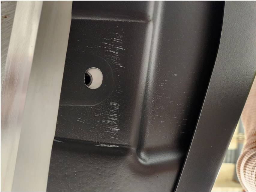
Figure 5.11: The offset between the plastic bumper in black and the aluminium FUP in silver. Note that the threaded hole cannot be fully seen through the bumper's hole
