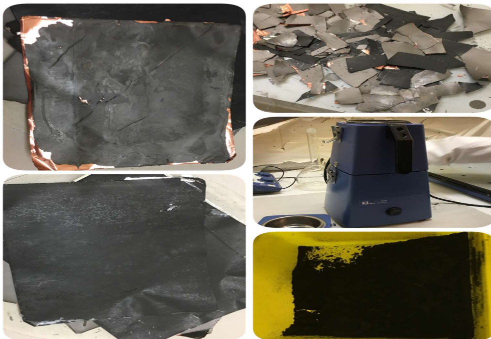
Figure 9: Sheets of cathode and anode from spent car lithium-ion battery. The battery is cut into small pieces and mixed to powder.
