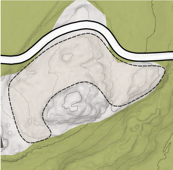
An appropriate site for a village is of low agricultural use, not too rough terrain, and close to existing connections.
