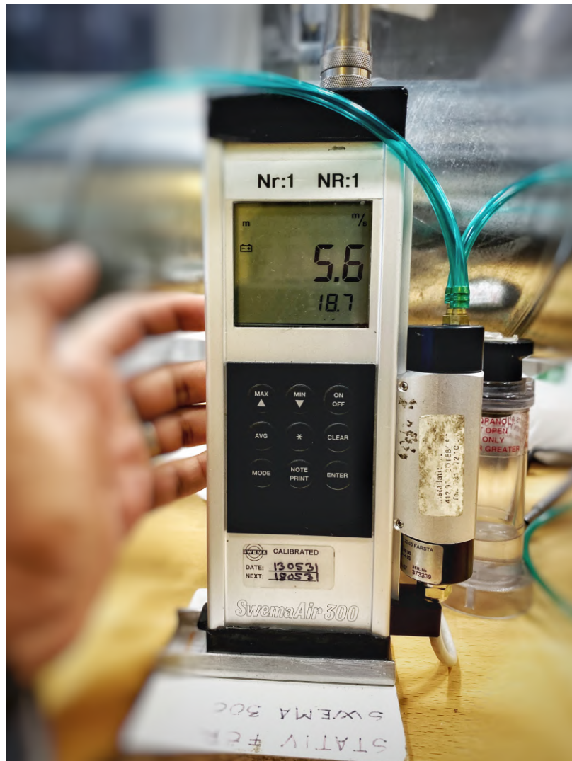
Figure 4.9: Air velocity and pressure differential instrument type Swema Air 300.
