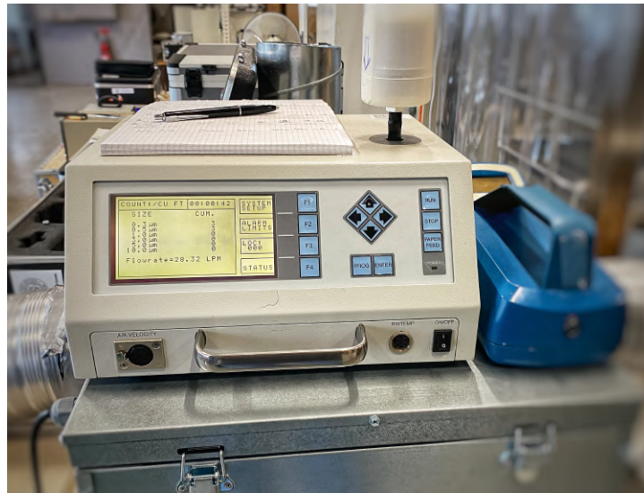
Figure 4.7: Optical particle counter (Met-One)
