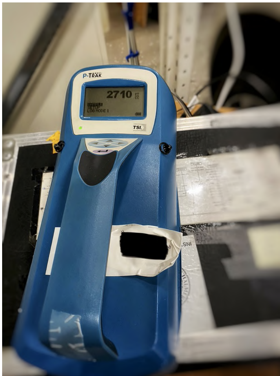
Figure 4.6: Condensation particule conter (P-Trak)
