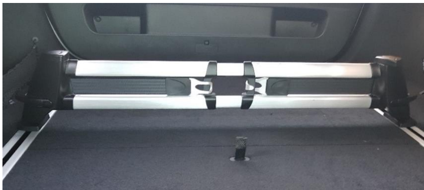
Figure 12 Trunk splitter with guide rails
