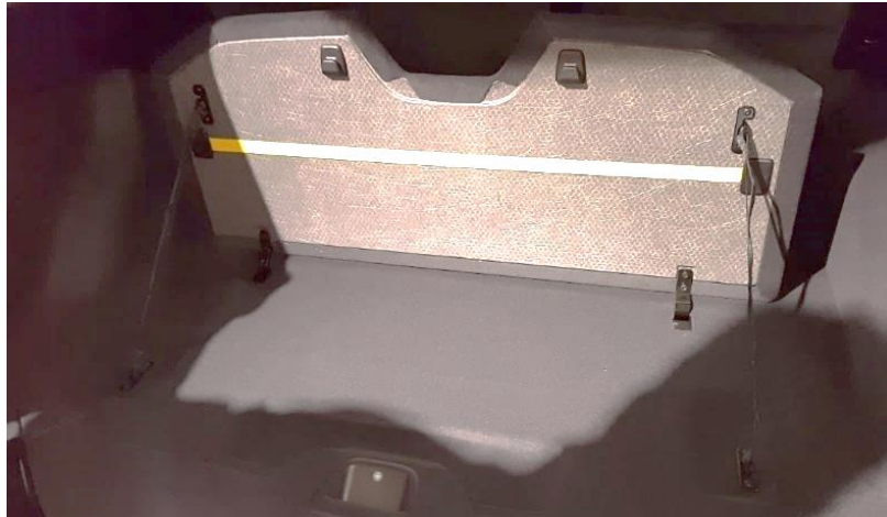
Figure 15 Integrated trunk splitter in Volvo V60
