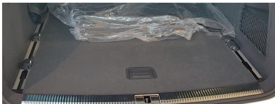
Figure 13 Trunk load floor with guide rails
