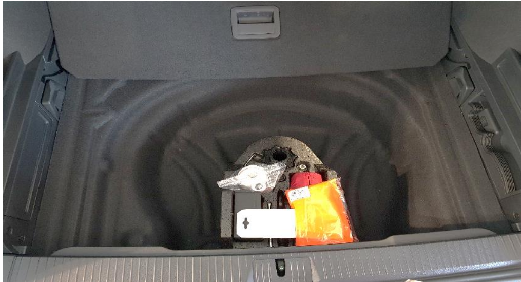
Figure 14 Tool storage space under the load floor
