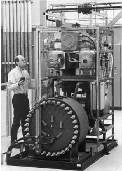
(a) 26 kW electrolyzer used in the PHOEBUS demonstration plant [65].
