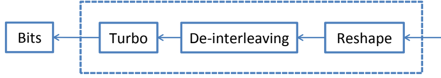
Figure 3.8: The structure of decoder is shown in the picture. Received slots will be reshaped and de-interleaved, and then send to Turbo decoder. Decision is made inside Turbo decoder, and decoded data bits are sent as output.
