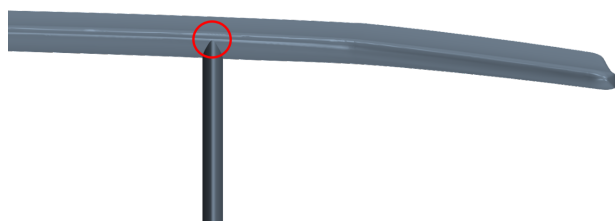
Figure 4.5: Position of the left pylon (24cm length) along with reference point, from -X axis
