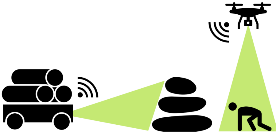
Figure 2.2: Drone aiding autonomous machine in detecting a hazardous situation from an additional point of view. [57]
