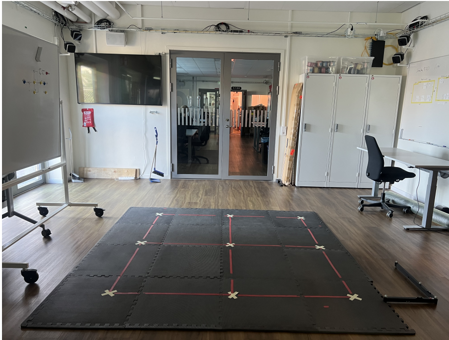
Figure 3.3: Lab environment setup: the robots will work on the black mats, MOCAP cameras can be seen on the top left and top right in the picture.s
