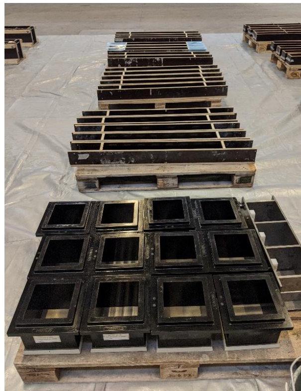
Figure A.2 Prism and material testing forms prepared for casting.
