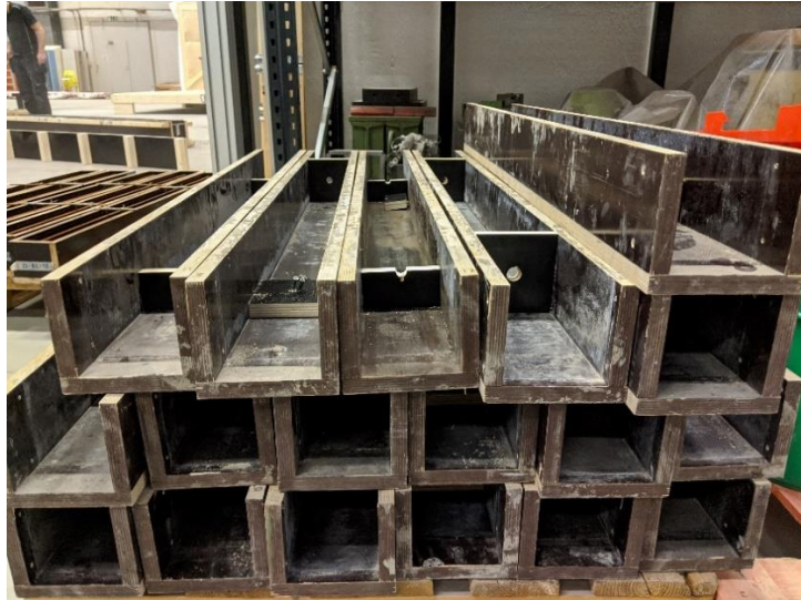
Figure A.1 Construction of reinforced prism forms.
