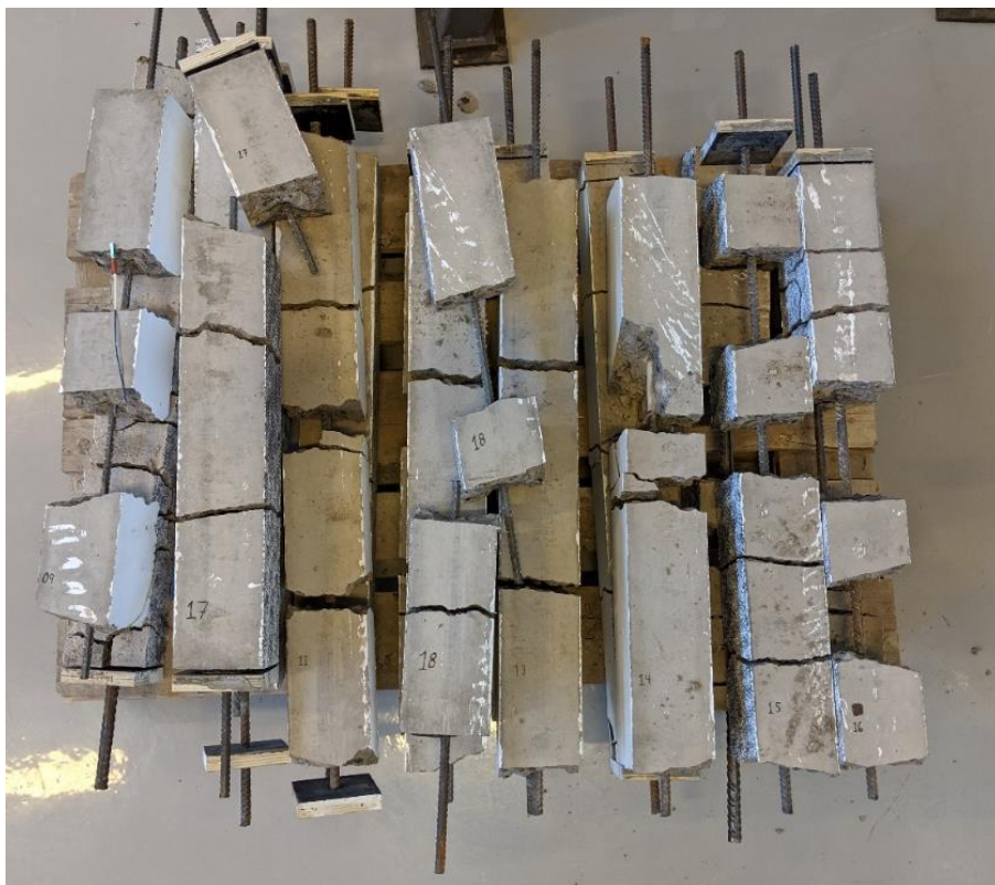
Figure A.12 Reinforced concrete prisms post-testing.
