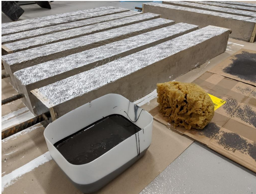
Figure A.7 DIC preparation including application of a white backdrop and a black speckle pattern.
