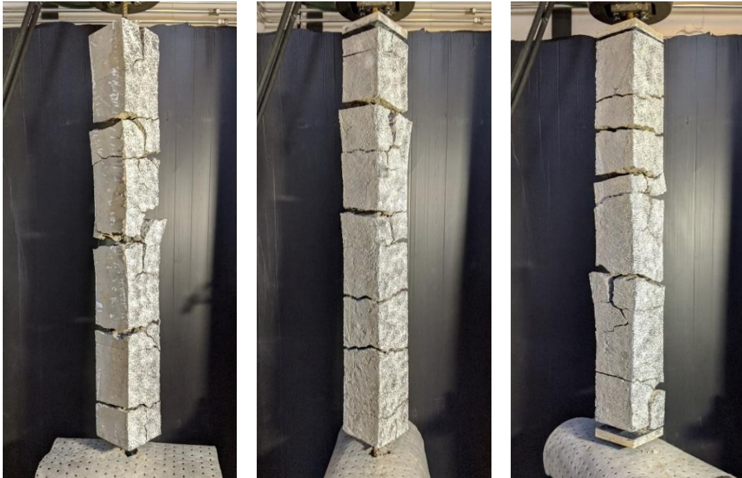
Figure F.2 Prism \phi 12 -5 (left), \phi 12 -11 (center), and \phi 12 -12 (right) post-testing.
