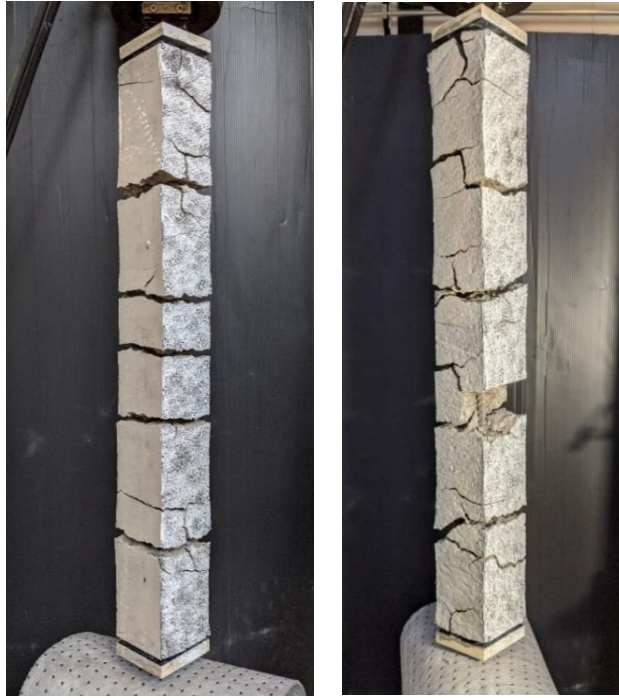
Figure F.1 Prism \phi 16-1 (left) and \phi 16-2 (right) post-testing. Note that an image of prism \phi 16-3 was not taken and is therefore not included.
