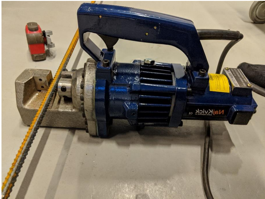
Figure A.3 Cutting of steel reinforcement for the prisms and material testing.
