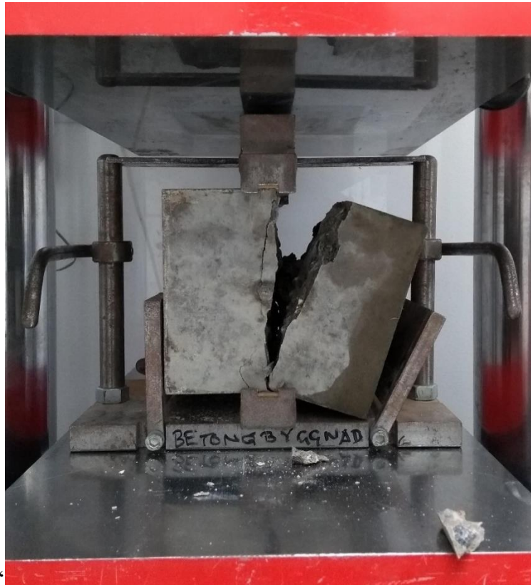
Figure A.13 Split testing concrete cubes.
