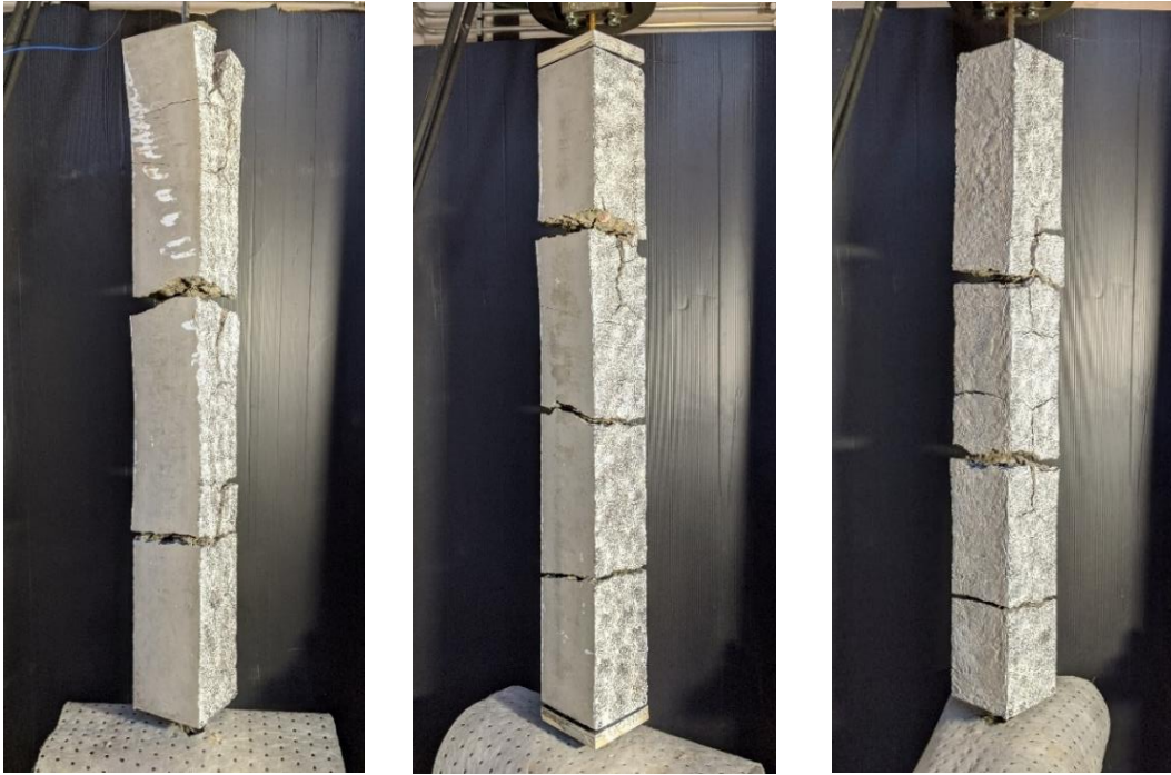
Figure F.6 Prism \phi 10-1 (left), \phi 10-2 (center), and \phi 10-3 (right) post-testing.
