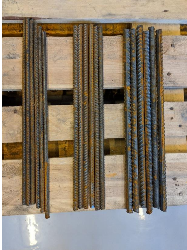
Figure A.9 Segments of steel reinforcement for material testing.
