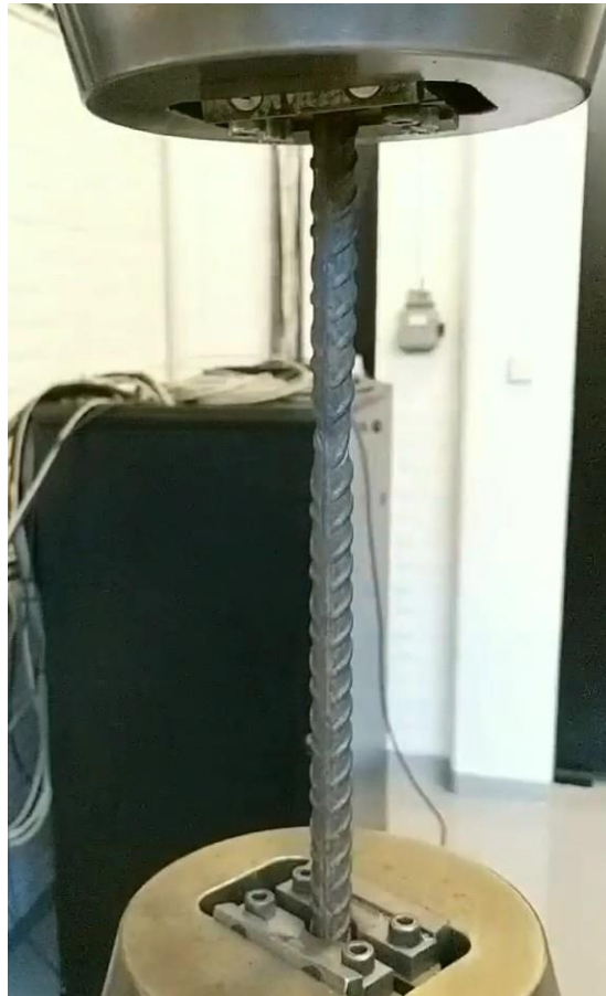
Figure A.11 Example of necking prior to failure in steel reinforcement.
